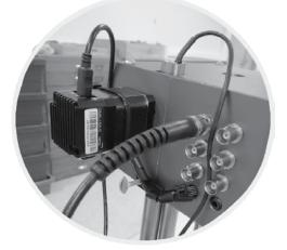
\*USB motor-drive (mains or battery) \*Load-displacement synced to micro-imaging \*Robust worm-gearing virtually eliminates backlash \*Range of load cells & displacement devices standard
